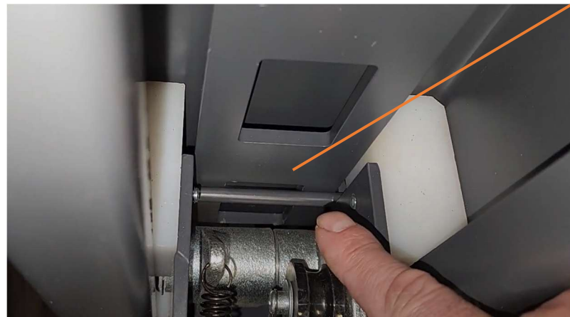
Safety Ladder inserted
