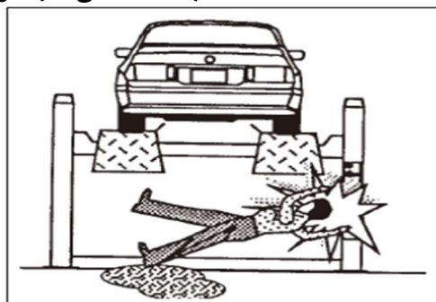
Figure 35 - Slip and fall risk
