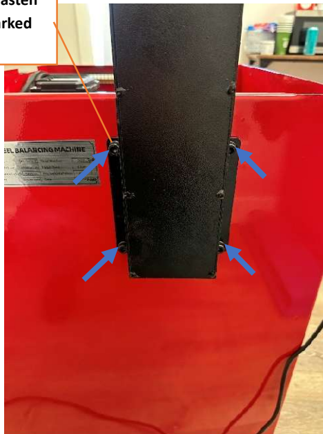
Figure 2.5 Removal and installation of the display panel support tube.
