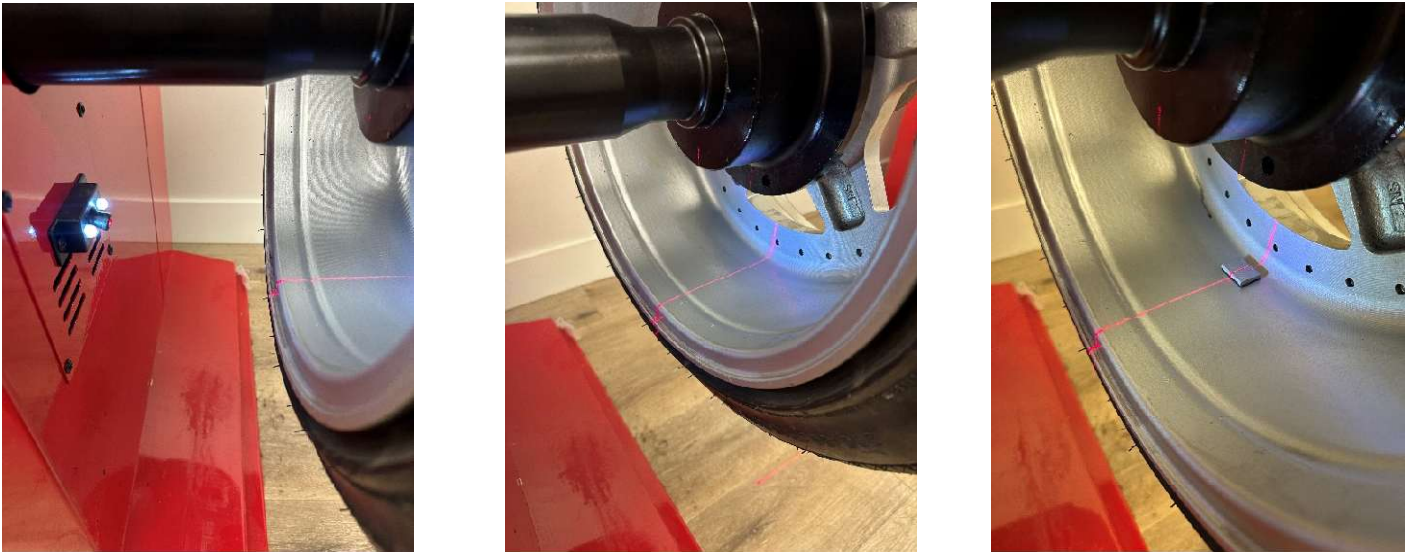
Figure 3.8.1 Balance block installation 6 o'clock position
