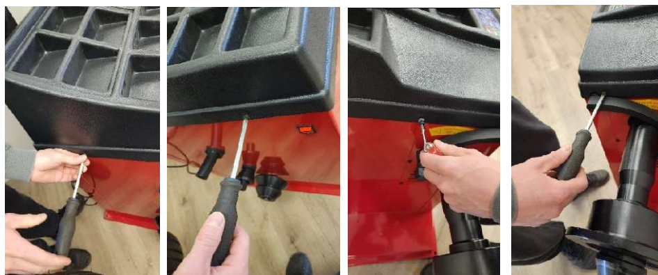
Figure 2.8 Installation of the top cover screws.
