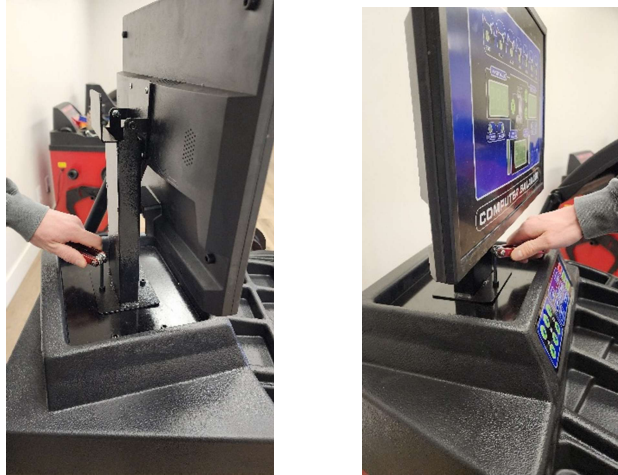
Figure 2.1 Secure the display panel to the balancer
