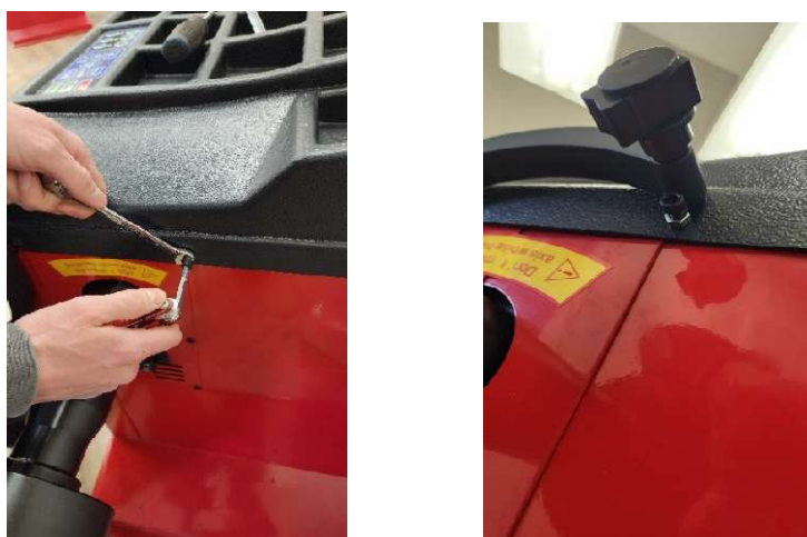
Figure 2.9 Installation of the support arm screw.
