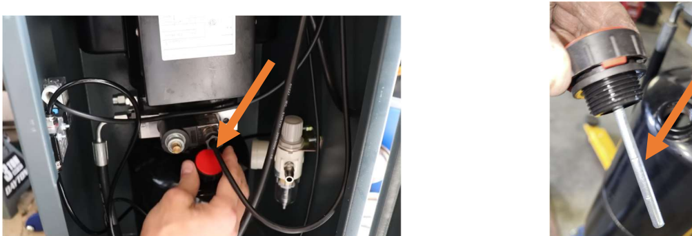
Figure 10: Hydraulic Reservoir Fill Port and Fill Level Mark
